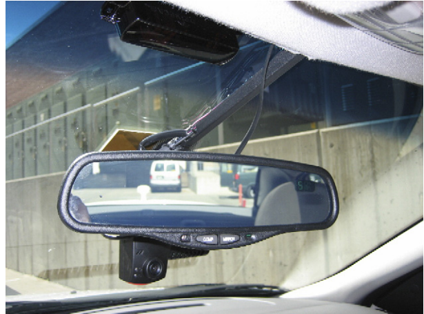
Fig. 1. View of the DriveCam event triggered video system located behind the rear-view mirror.
